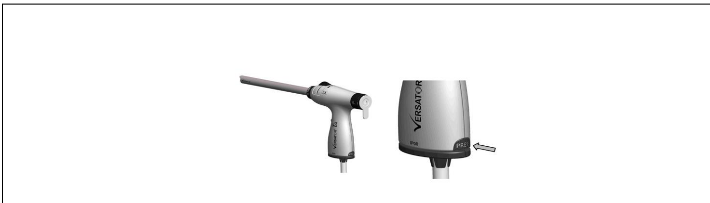
Figure 10: “Press” button provided at the lower end of the Handpiece
